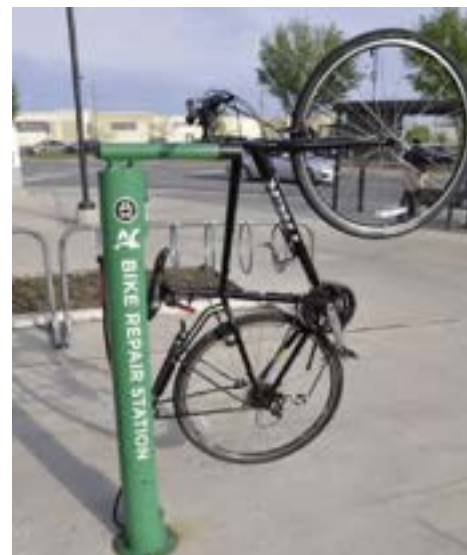
Bike Repair Stations allow cyclists to mount their bicycles and use the provided tools to perform minor repairs.
