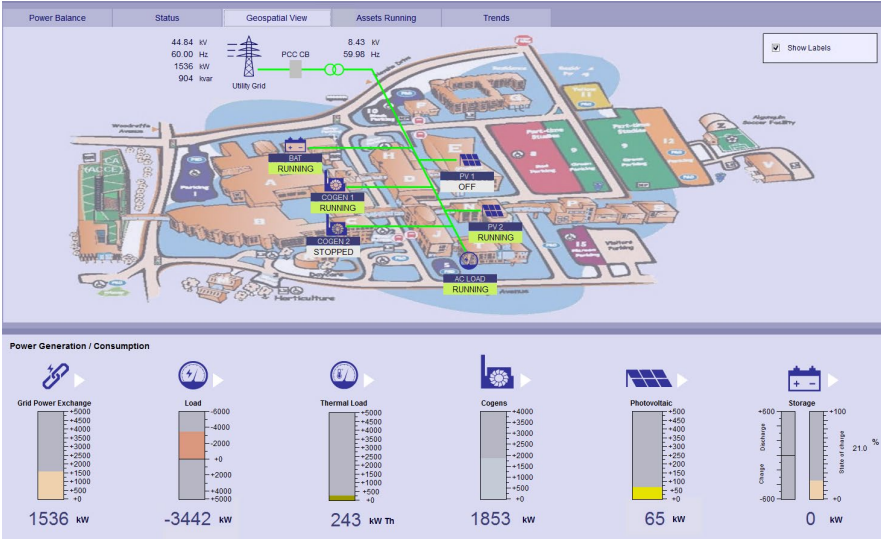
Figure 1 Microgrid Geospatial View and Operations Status
